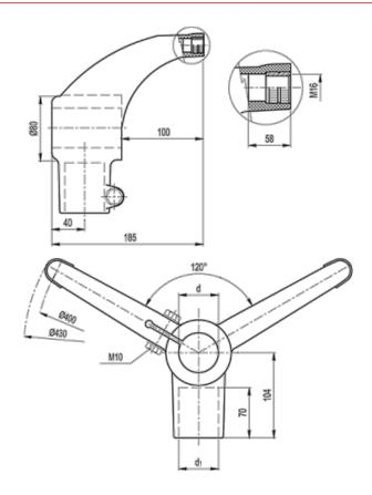
d (inch) = 2 Gas d1 (inch) = 1 1/2 Gas d1 (mm) = 48.3 d mm = 60.3 Weight (g) = 700
